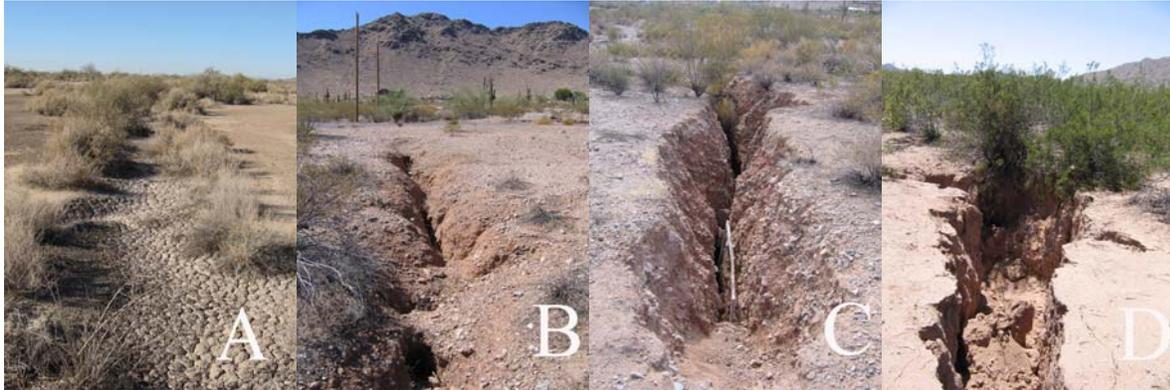
**Figure 2. Earth fissures interior geometries are grouped into four categories. A) Rounded edges with a flat bottom, B) rounded edges with a crack bottom, C) sharp edges with a crack bottom, and D) sharp edges with a flat bottom.**
