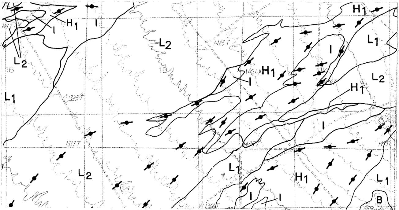
b) Geologic flood-hazard map of the same area. Heavy dots with lines show approximate locations of channels of major drainages that head in adjacent mountains. Surface age, proximity to major drainages, local topographic relief, and evidence of channelized flow were used to delineate flood-hazard zones. See text for description of flood-hazard categories.
