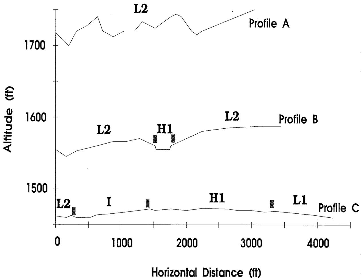
Figure 1. Topographic profiles showing changes in the extent of flood-prone areas downstream and away from the mountains. Profiles were constructed perpendicular to a large stream draining the western side of the White Tank Mountains. Flood-hazard zones are discussed in the text.
