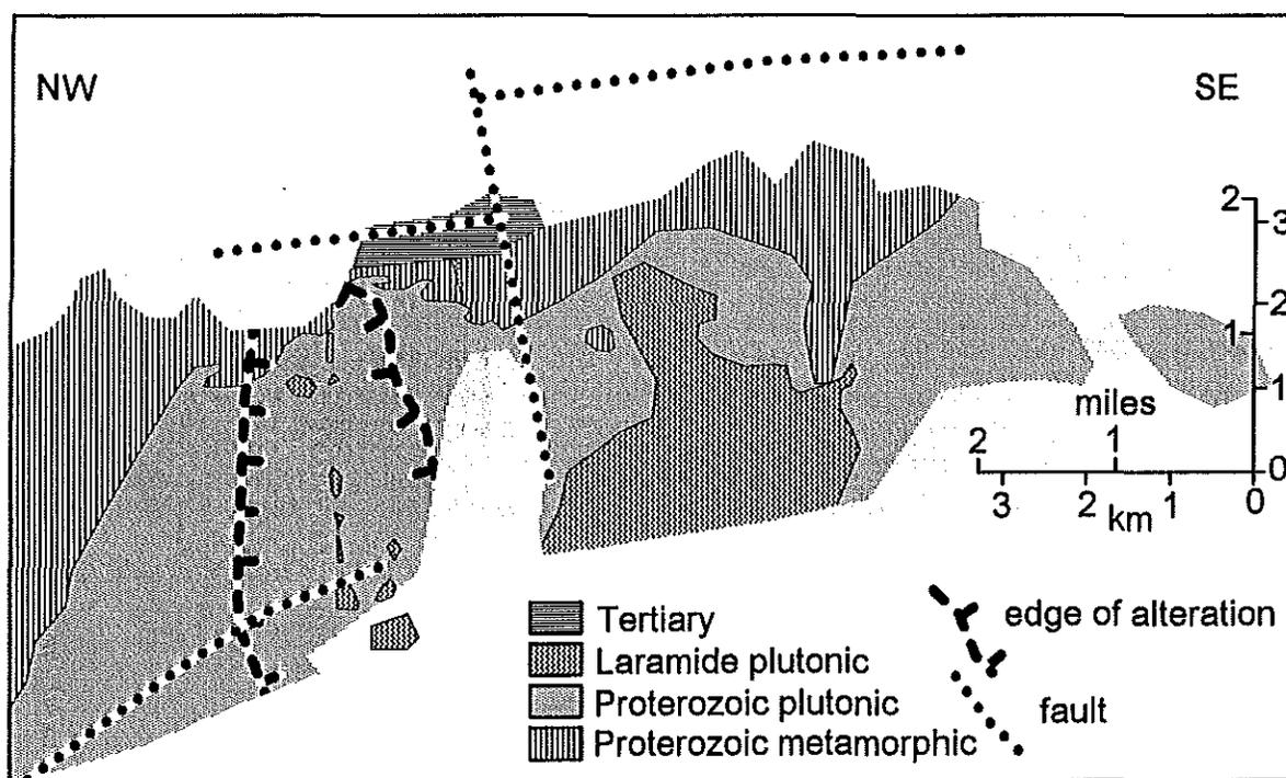
**Figure 1** Schematic right section striking  $150^\circ$ , dipping  $40^\circ$  to the southwest drawn through Comode Butte, eastern Santan Mountains. Blank areas depict areas covered by alluvium. Faults bound areas that were treated as undeformed blocks tilted  $50^\circ$  to the northeast. Geology was restored across the fault zones based on surface information. Note the classic porphyry copper alteration halo that occurs around the Mineral Butte area.
